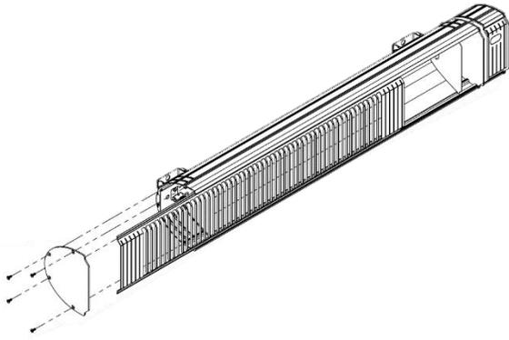
5. Carefully slide the protective grille out of the heater body to expose the emitter and the plastic sealing connectors.
