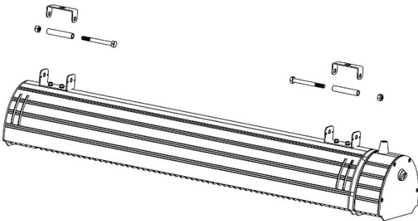
3. Install the two wall mount pivot brackets using the screws removed in the previous step.
