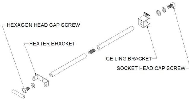
2. Secure the heater to the mounting brackets using nuts and washers provided.
