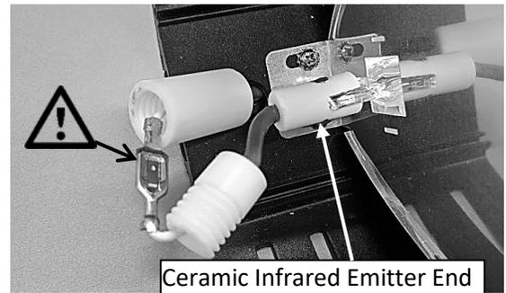
7. Bend the metal tabs to remove the small reflector shield sheet metal parts. Hold on to these pieces. This will allow you to slide the emitter into a bigger cavity to remove it from the reflector and heater body. Properly dispose of the broken emitter at your local recycling center.
