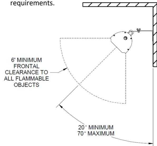
The angles of attachment are 20° to 70°, measured from the mounting wall.
