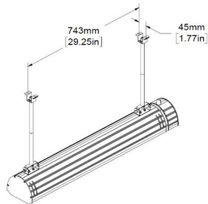
5. The heater can be hung vertically or pointed at a maximum angle of 45° from vertical.
