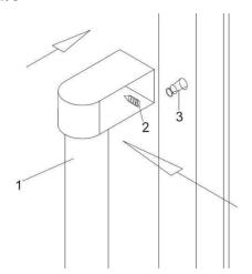
Locate the handle(1)over the pins(3)of the door and tighten the handle by screwing the Allen key grub screws(2)
