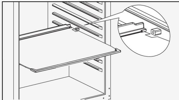
For easy access to the storage content, you must pull the shelves approximately 1/3 out of the rail compartment.
