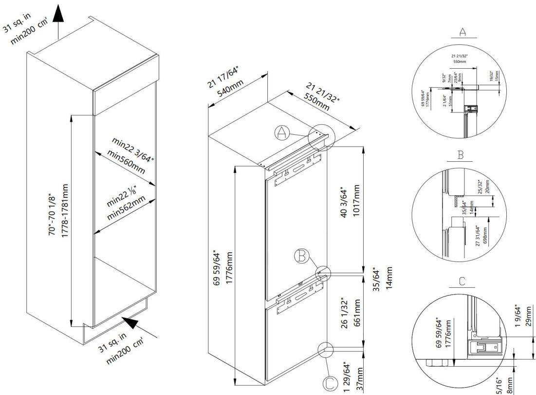
An air intake should be provided somewhere in the cabinet run to allow free air in. In this example, a plinth vent is shown underneath the refrigerator.
