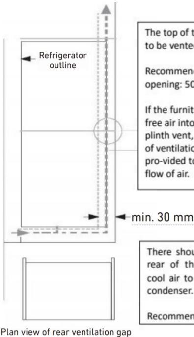
The open channel at the rear is clearly shown. For the correct operation of the appliance it is important that the top of the housing unit is not blocked off. A channel depth of 1 37/64" - 1 31/32" (40-50mm) is normal with most units.
