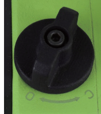
Image 2: Gas ballast shown in "open" position
