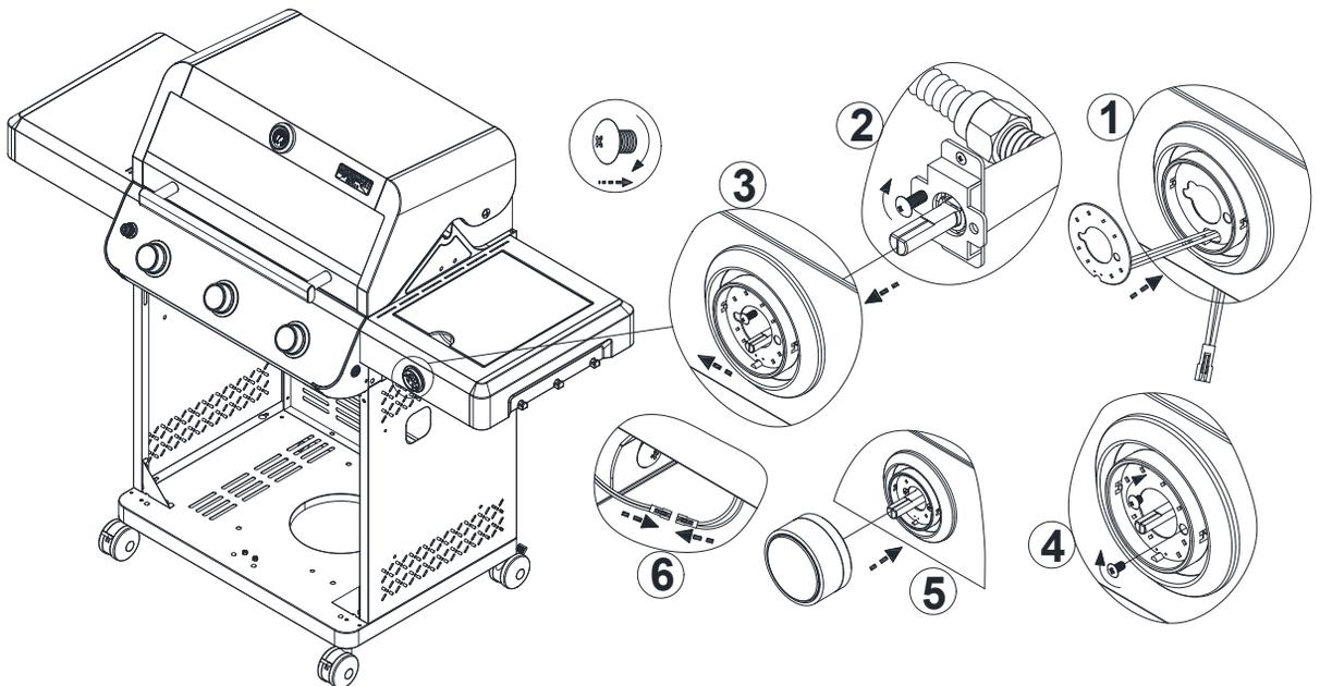
1. Insert Side Shelf, Right, LED Lamp Panel and Control Knob as the figure shows.
