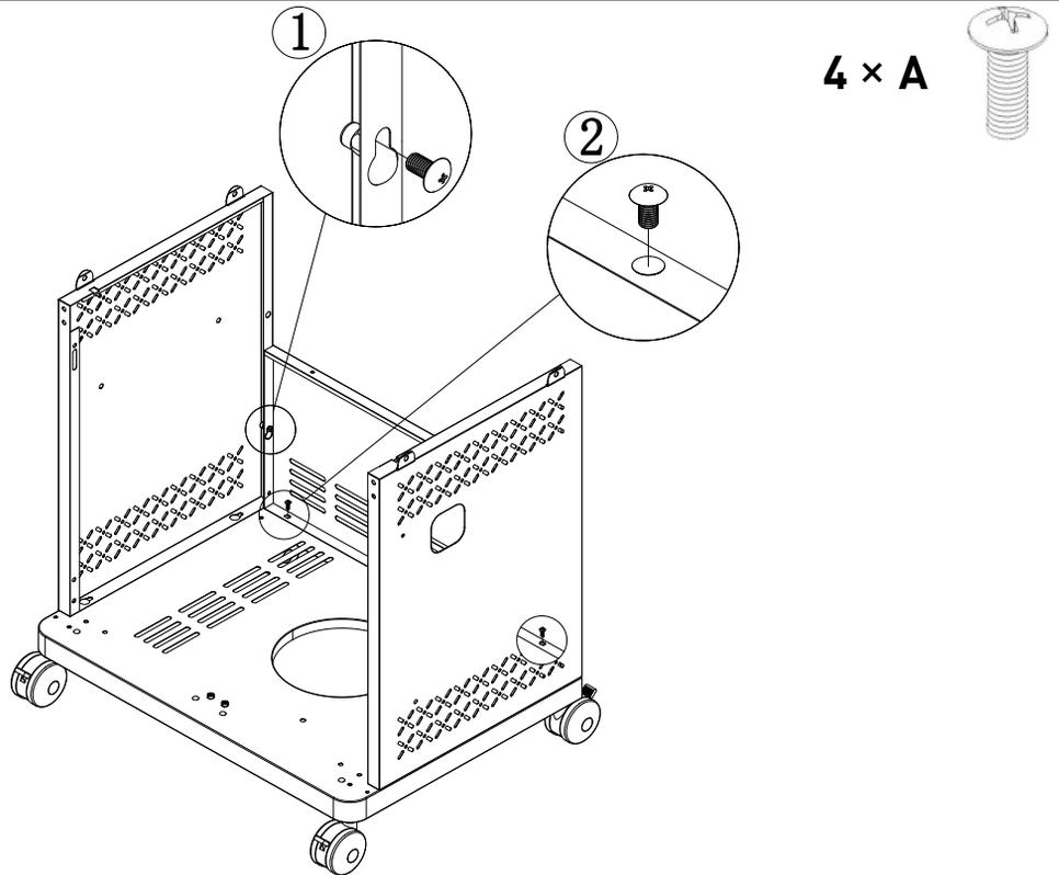
Install Cart Back Panel onto the relevant place with four A screws.
