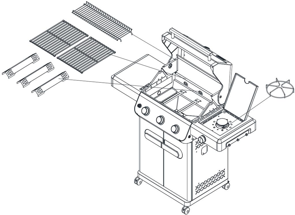
Put Warming Rack, Cooking Grid, Flame Tamer into the relevant place.
