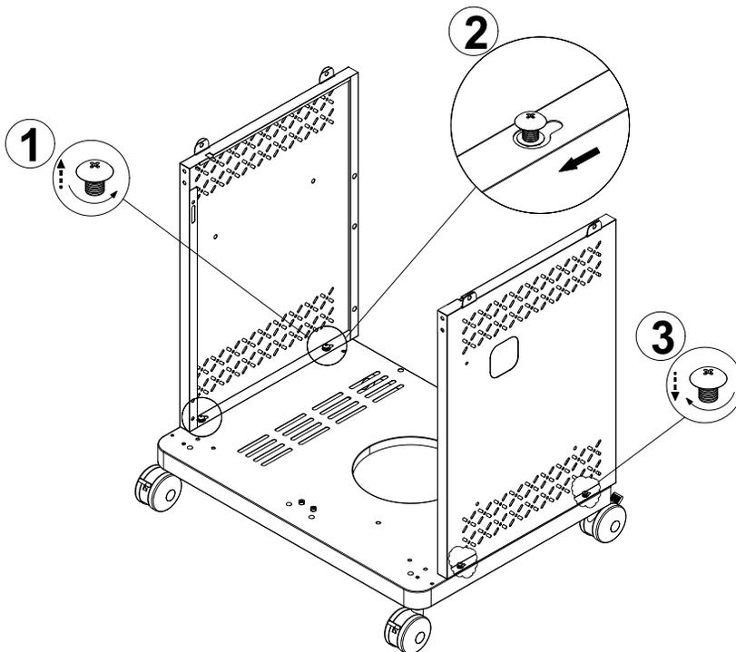
Half screw out the screws in the bottom plate, then put Cart Right Side Panel and Cart Left Side Panel onto the relevant screw holes and screw tightly.
