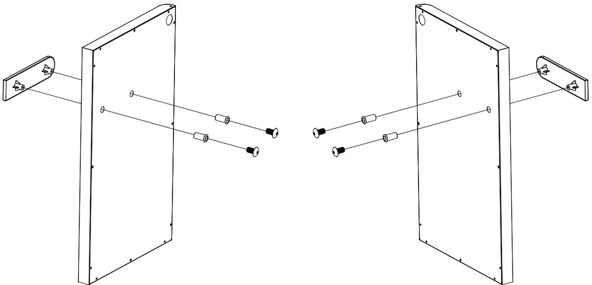
Install the Door Handle onto the Cabinet Door.
