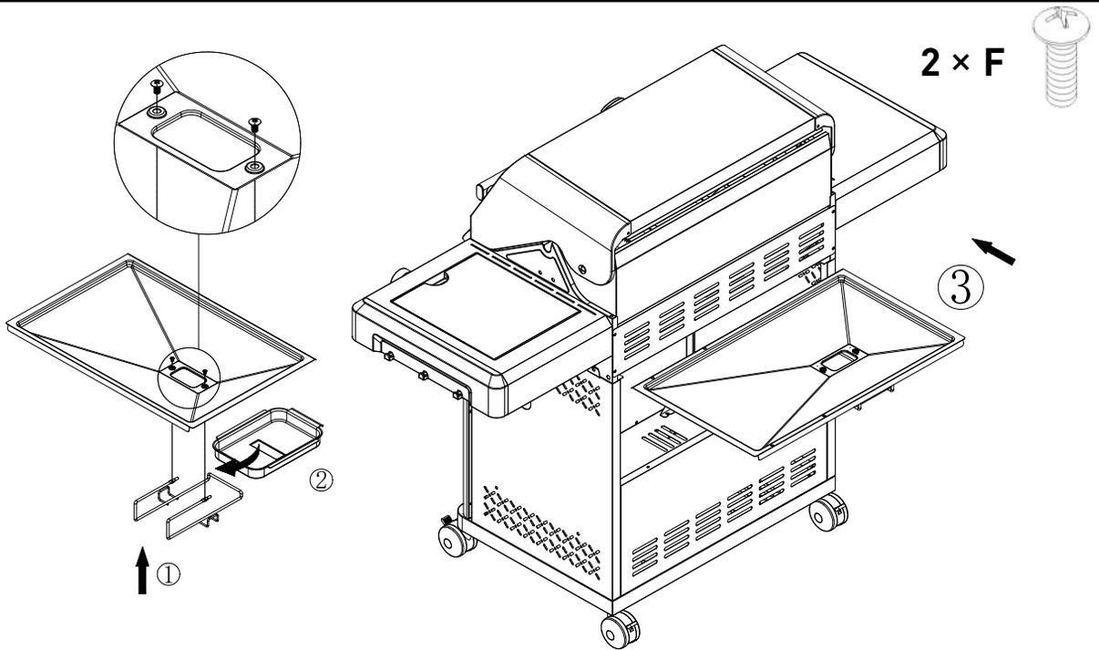
1. Install Grease Tray onto Grease Pan Bracket with two F screws.
