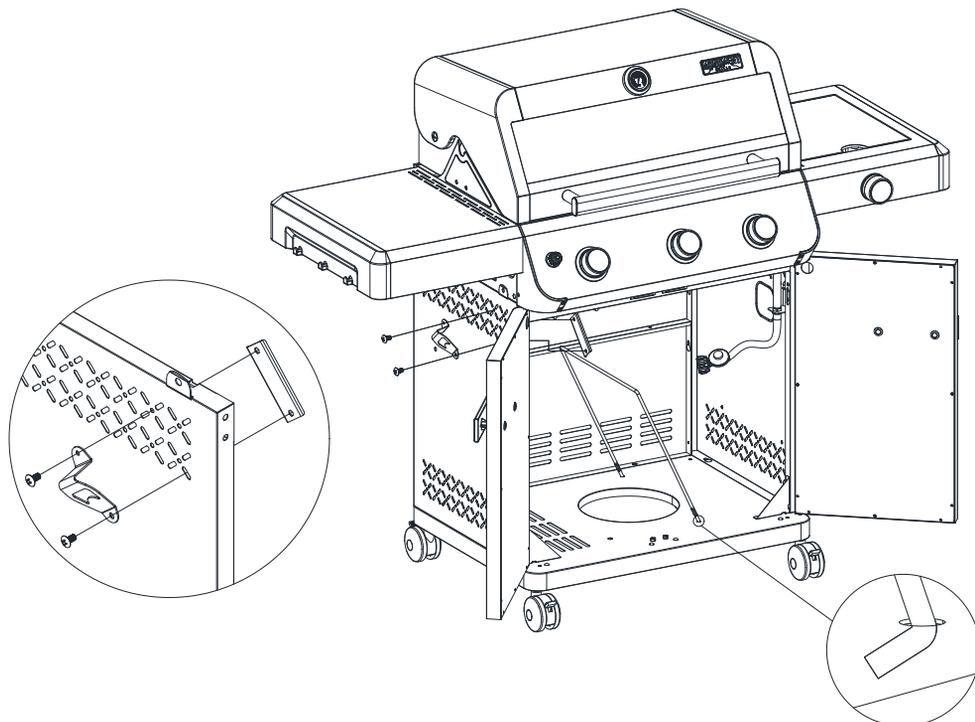
Install Gas Tank Holding Wire onto the bottom plate.
