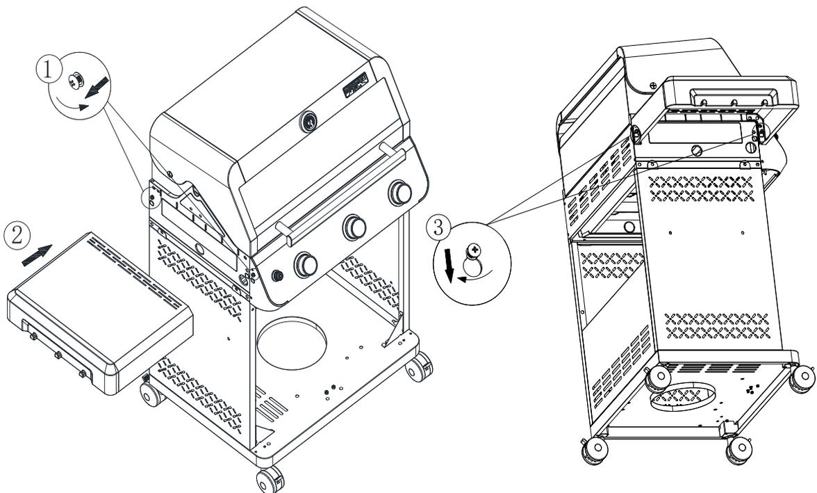
Half screw out the screw in the grill body, then put Side Shelf, Left onto the relevant screw holes and screw tightly.
