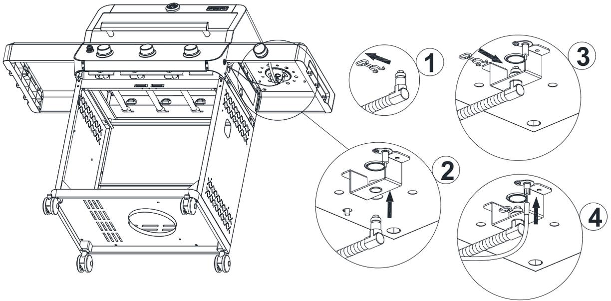
Half screw out the screw in Side Shelf,Right, then put it into the hole and screw tightly.
