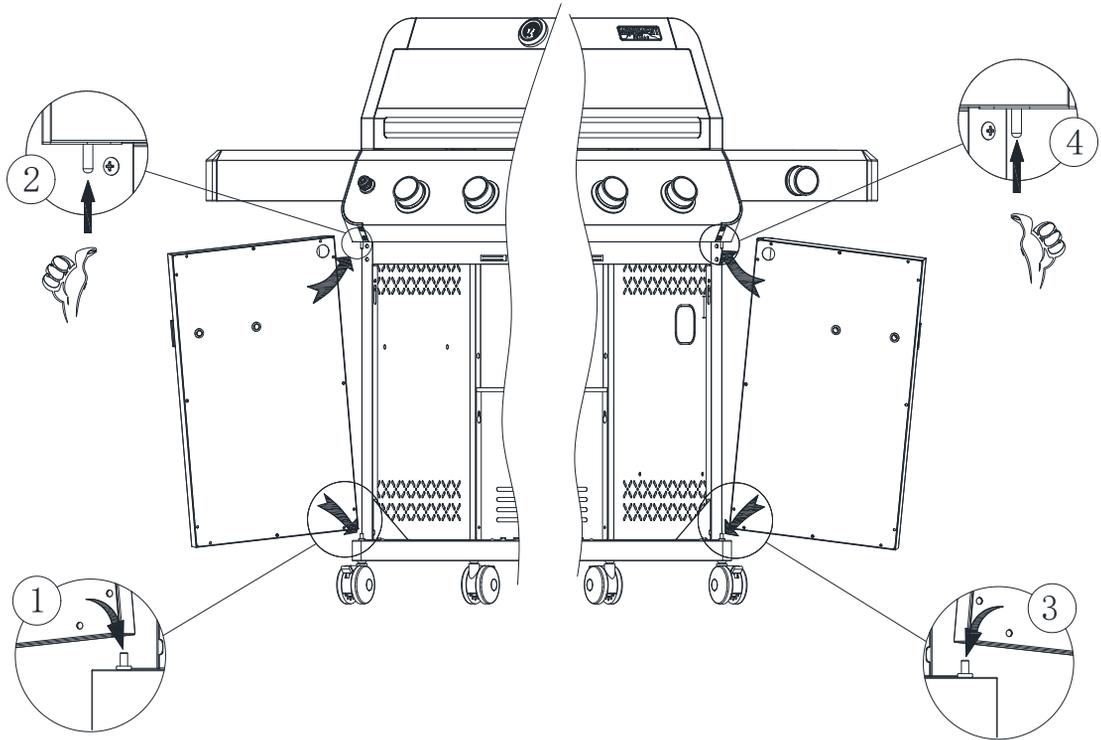
Install the Cabinet Door onto the Cart Bottom Board.
