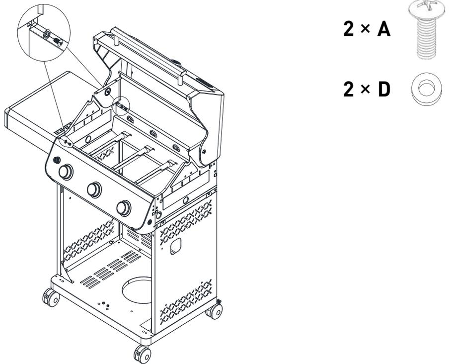
Install Side Shelf, Left onto grill body with A screw and D spacer.
