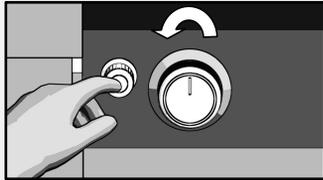
7. If the burner does not light after 5 seconds, turn knob to OFF. Turn gas OFF at LP tank and wait 5 minutes for gas to clear. Then turn gas ON at tank and repeat step 6.
