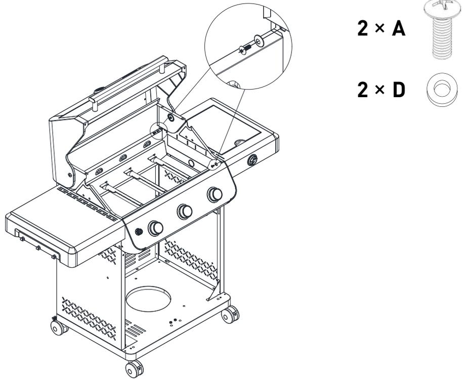
Screw Side Shelf, Right tightly with A screw and D spacer inside the grill body
