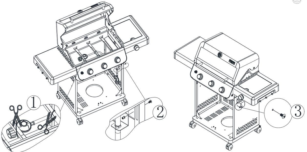
Fixed Regulator connecting piece onto the Right plate with one F crew.
