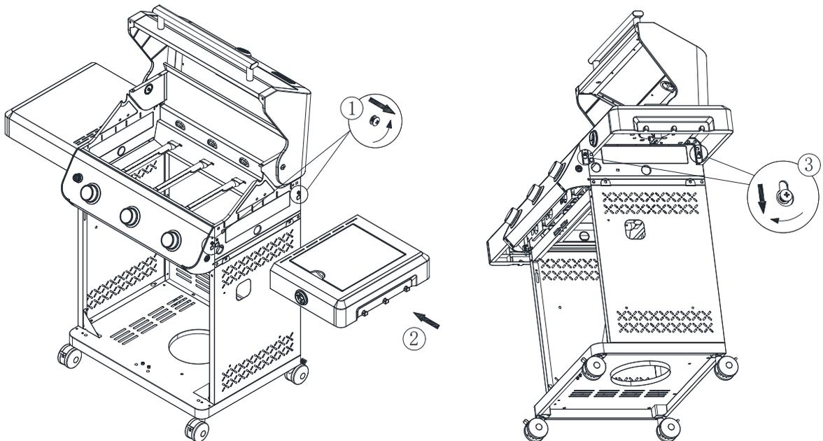
Half screw out the two big screws outside the grill body, then put Side Shelf, Right onto the relevant screw holes and screw tightly.
