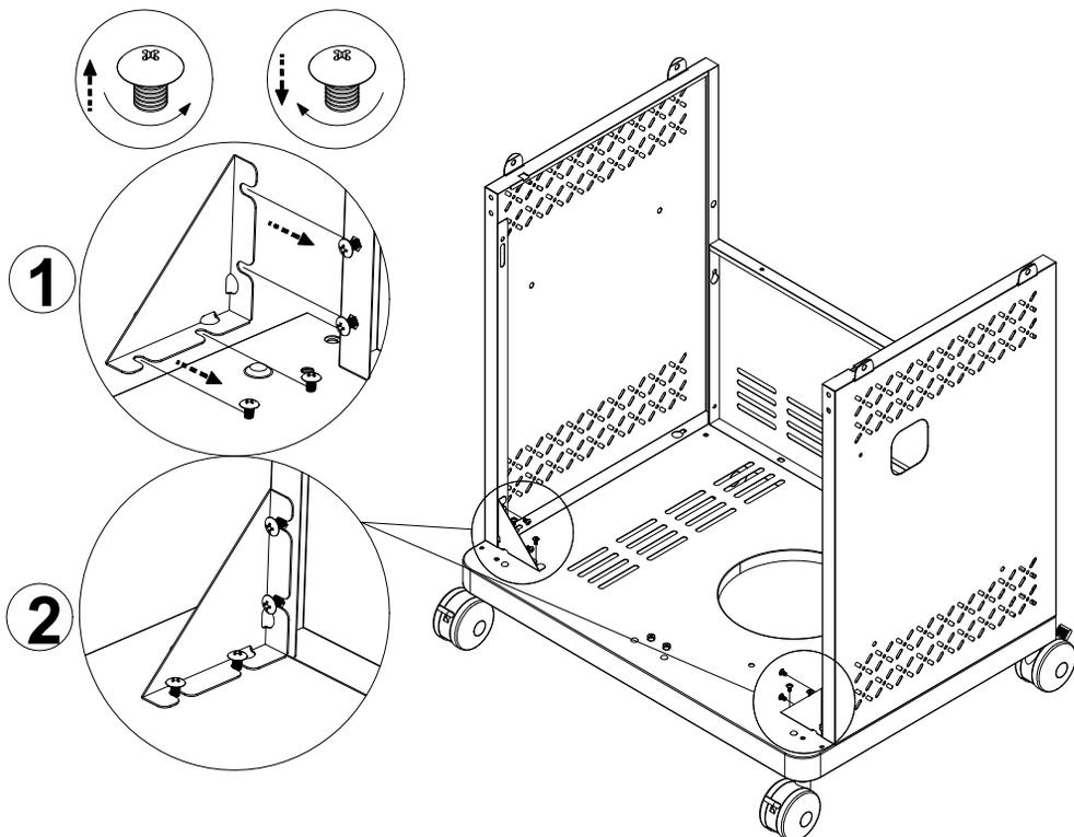
Half screw out the screws in the bottom and side plates, then put Triangle Joint Parts onto the relevant screw holes and screw tightly.
