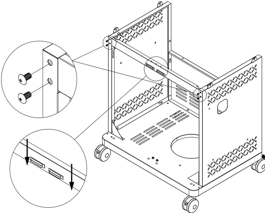
Install Cart Front Bar onto the relevant place with four F screws.
