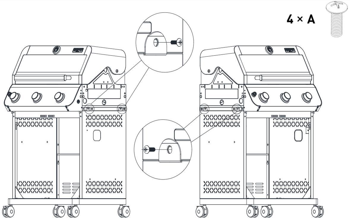
Screw the grill body and the cart tightly with four A screws.
