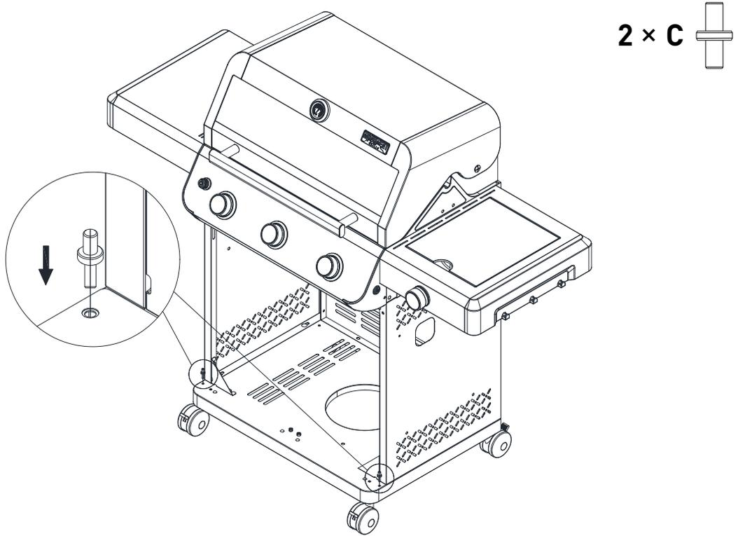
Put the Spindle Below Door Panel into the relevant hole in the bottom plate.
