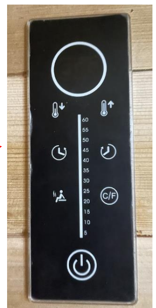
Sauna Control Panel has no Illumination
