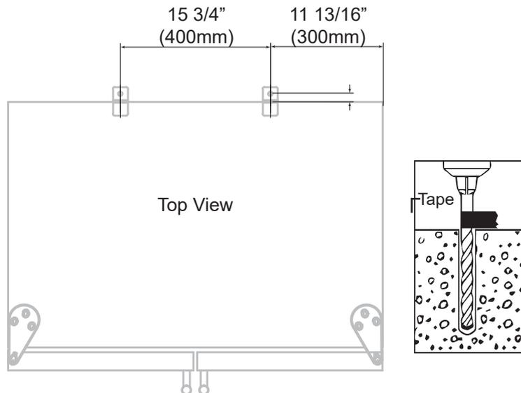
*TIP: Use painter's tape to judge how deep of a hole you are drilling. First, cut a piece of painter's tape several inches long. Then, place the tape on your drill bit at the depth of the expansion bolts shield to drill. Once you reach the tape, you know when to stop drilling. Don't drill too deep.*
