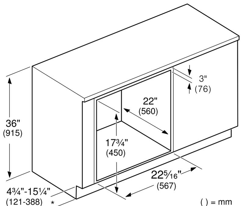
**NOTICE:** The cabinet base must be flat and capable of supporting a weight of at least 142 lbs (64.1 kg).
