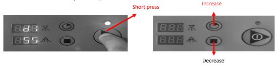
To save and exit the operator menu at anytime, press Confirm Button for 3 seconds.
