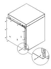
Make electrical connections according to wiring diagram supplied with the machine and secure wires to the machine service connection. Recommended wire specification as 4\*10AWG. Keep excess wire in the base of the unit to a minimum.
