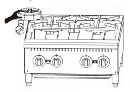
4.Replace the orifice fittings into the valveNote: Unit Number on side of orifice fittings
