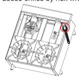
2. Raise the top burner and pull, Exposed the orifice.
